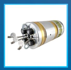
Positively isolate and monitor potentially explosive vapors during hot work, then hydrotest new weld connections with one simple to use tool. Dual port design creates a positive pressure barrier between the seals, safely isolating the hot work from any residual upstream gases.
